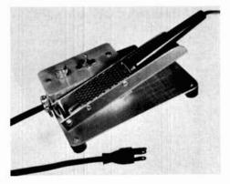
to the iron. Any power diode with a PRV rating of at least 300 volts will do. The diode is connected across the normally-closed terminals of a microswitch. When the iron is lifted for use, the internal spring in the microswitch operates, returning the switch to its closed position, shorting out the diode. Full power is then available to the iron (see fig. 2). A handy pilot light tells you that power is on and shows the effect of the series diode.
